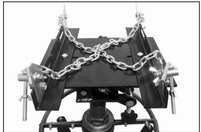
Figure 12. Chain attachment and platform adjustments.
