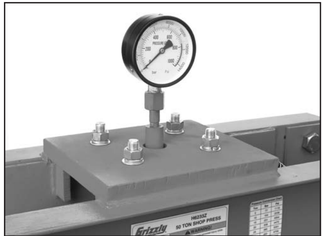
Figure 10. Pressure gauge installed.
