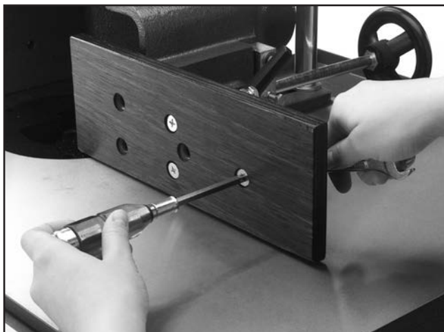
Figure 18. Attach wooden fence assembly.
