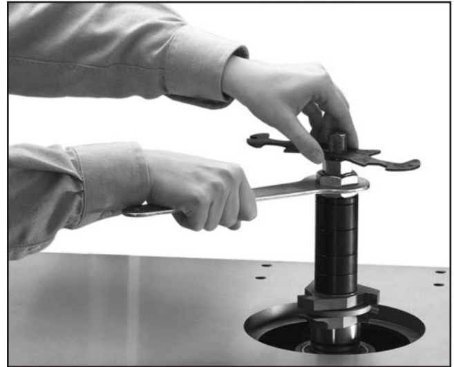
Figure 30. Tightening spindle nuts.
