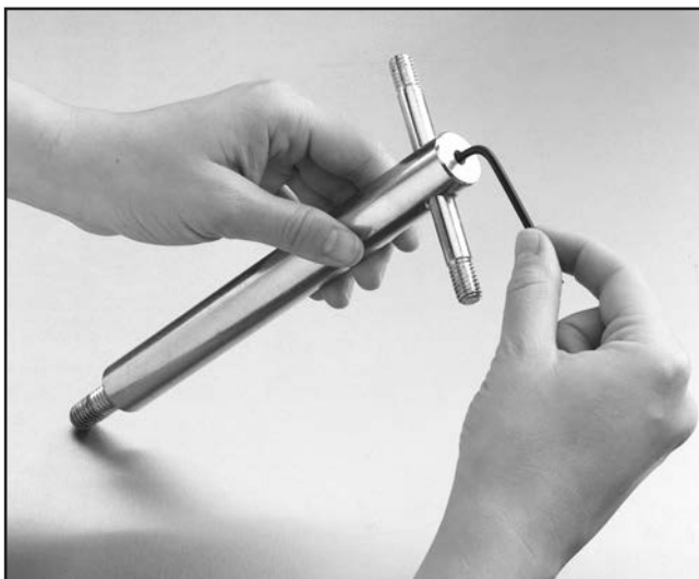
Figure 11. Tightening setscrew with hex key.
