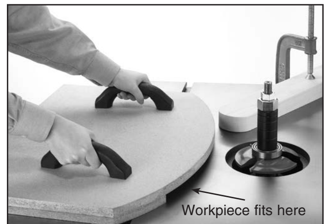
Figure 40. Pattern jig for making curved pieces.
