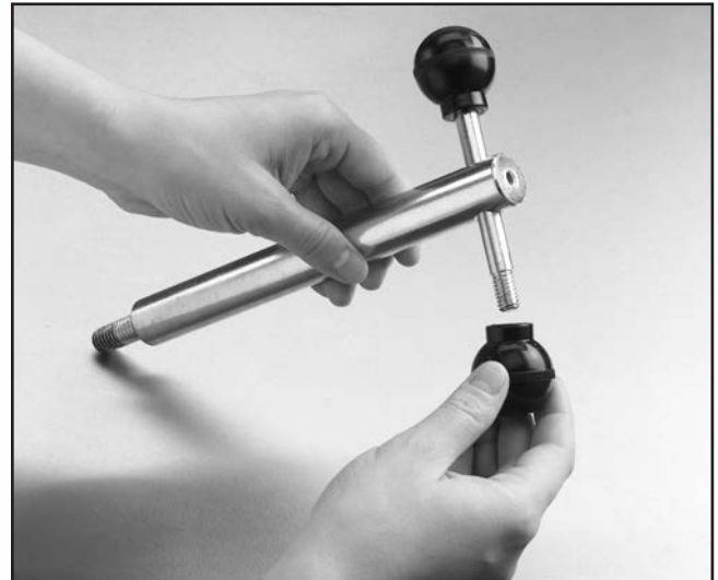
Figure 12. Round knobs onto bar.
