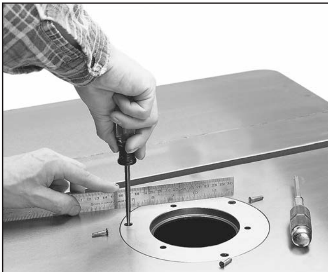
Figure 28. Leveling table insert.
