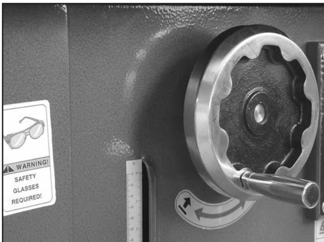
Figure 21. Handwheel mounted to shaper.
