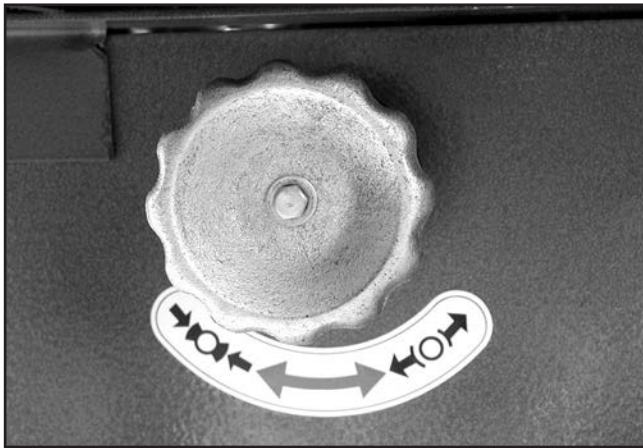
Figure 31. Location of spindle lock.
