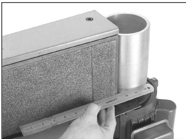
Figure 55. Example of checking bottom of platen-to-roller.
