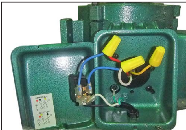
Figure 59. G1140 motor wiring (prewired 220V).
