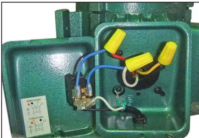
Figure 61. G1531 motor wiring (prewired 220V).
