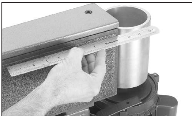
Figure 54. Example of checking top of platen-to-roller.
