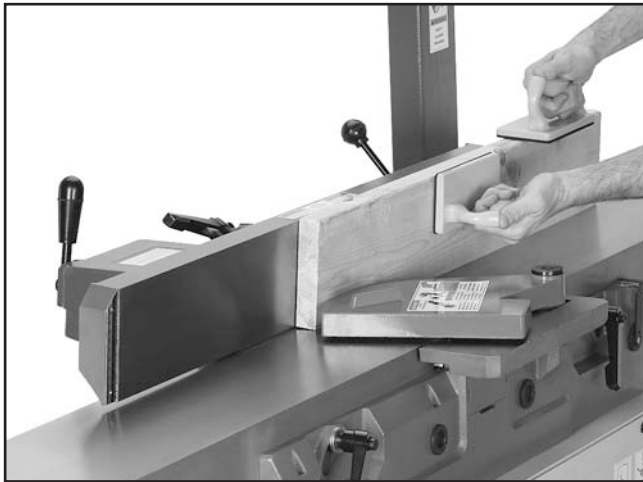
Figure 34. Typical edge jointing operation.
