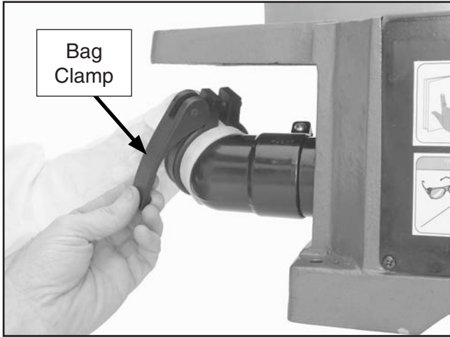
Figure 20. Attaching the dust collection bag.
