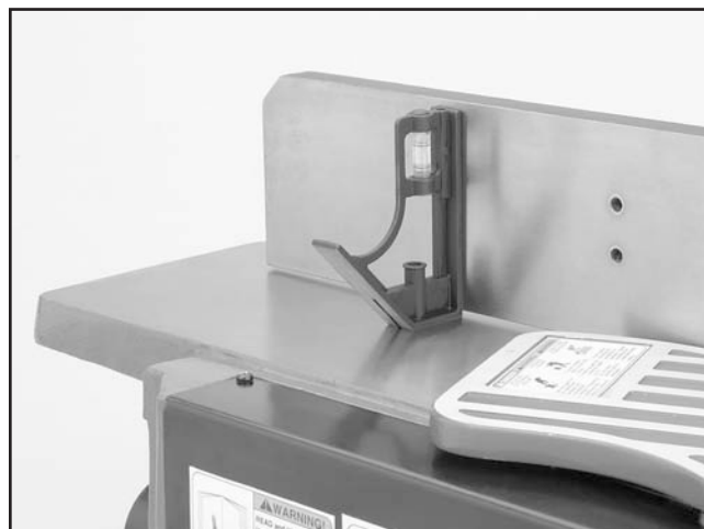
Figure 24. Checking the 90° stop.
