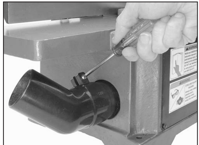
Figure 19. Installing the dust chute.
