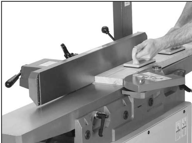
Figure 32. Typical surface planing operation.
