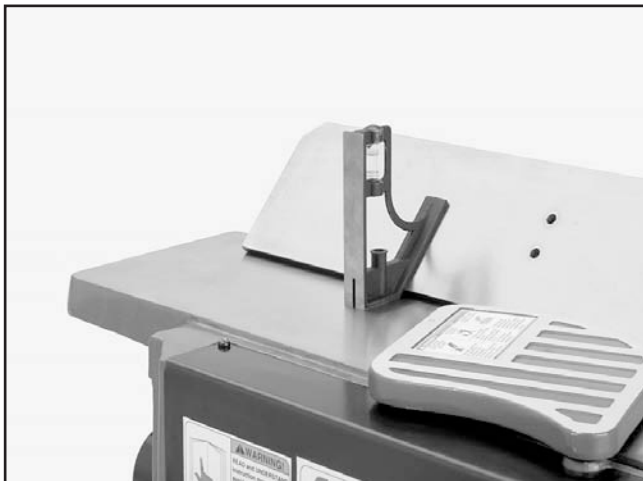
Figure 27. Checking the outward 45° stop.
