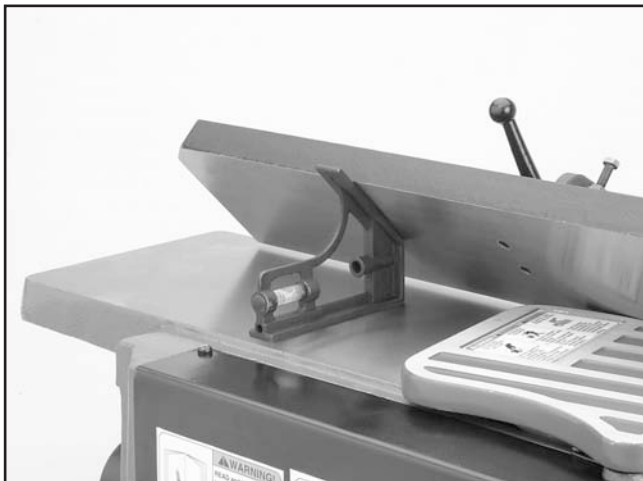
Figure 25. Checking the inward 45° stop.
