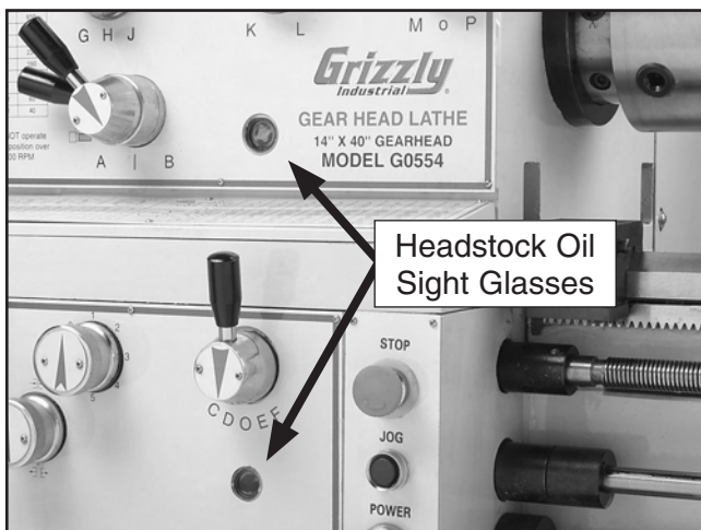
Figure 11. Headstock oil sight location.
