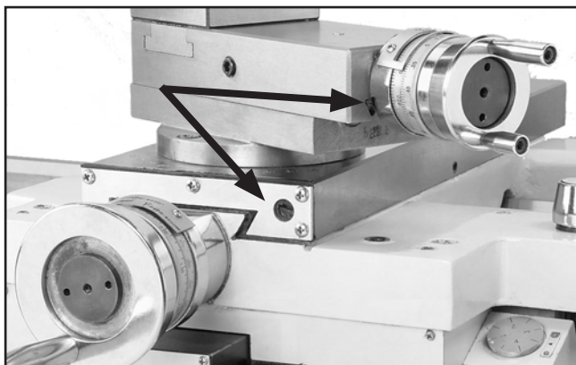
Figure 87. Front cross feed and compound rest gib screws.
