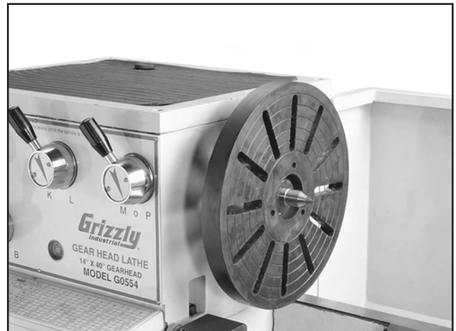
Figure 40. Typical faceplate and dead center setup.
