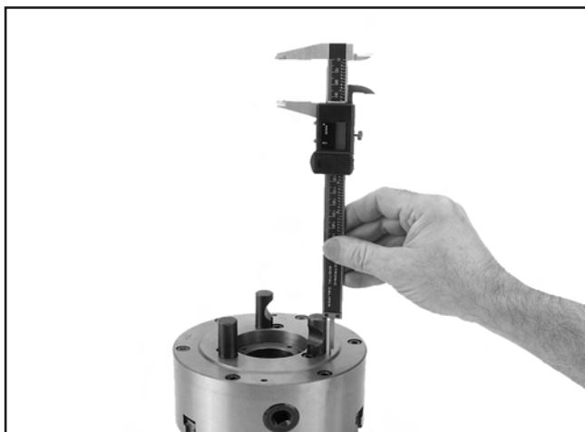
Figure 18. Measuring height of cam-lock studs.
