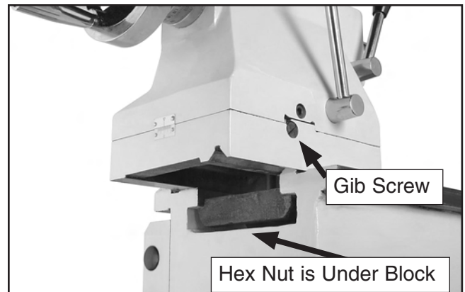
Figure 88. Tailstock nut and gib adjustment.
