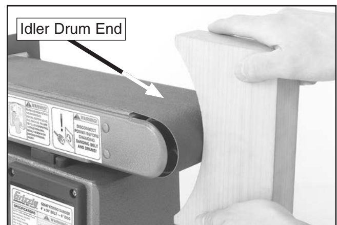
Figure 22. Sanding an inside curve.
