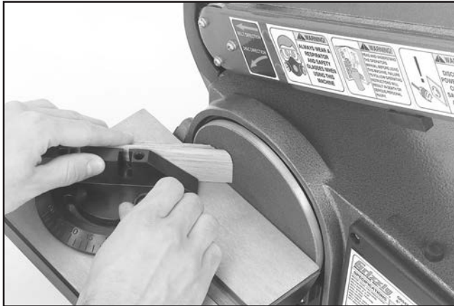
Figure 19. Angle disc sanding.
