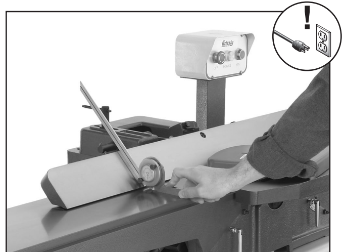
Figure 60. Example of adjusting fence 45° outward.
