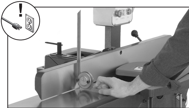
Figure 58. Example of adjusting fence to 90°.
