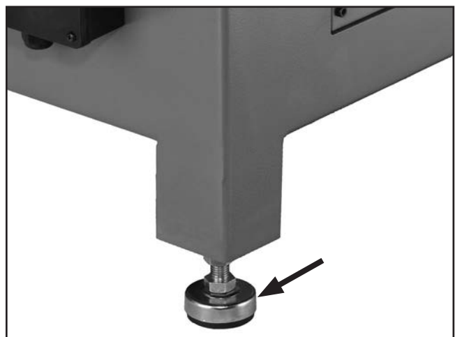
Figure 20. Foot installed in cabinet leg.
