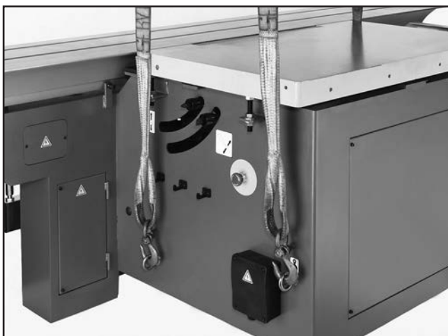
Figure 19. Lifting the saw base unit.
