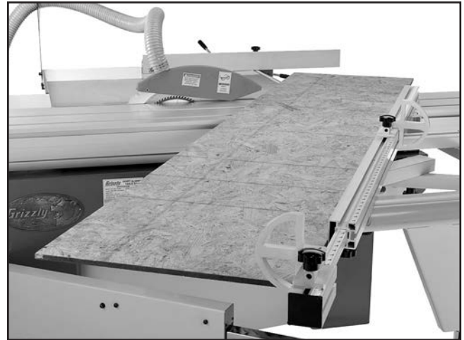
Figure 95. Example of miter cutting operation.
