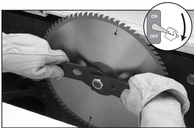
Figure 43. Installing the main blade.
