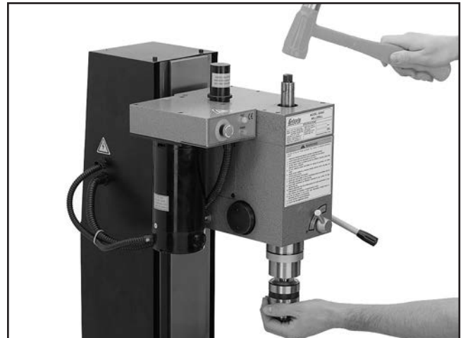
Figure 9. Striking the drawbar.
